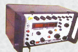
Secondary Injection Test
